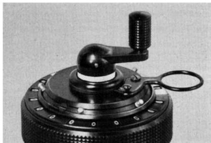
Fig. 5. Operating handle, extended axially for subtraction
